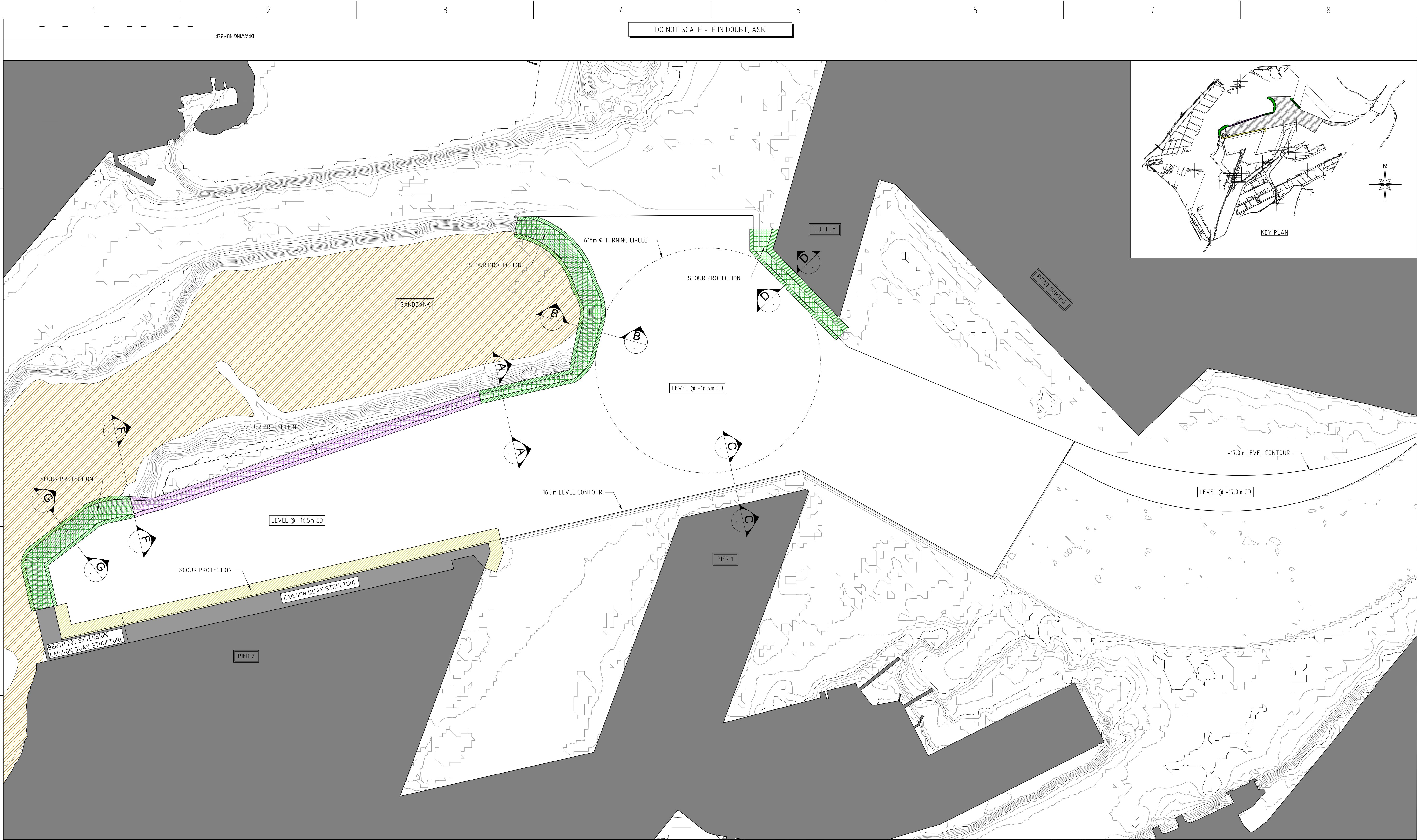
PLAN: SCOUR PROTECTION LAYOUT-OPTION 3 (CAISSON OPTION ILLUSTRATED)
